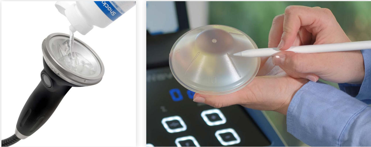
Figure 10 - Gel on transducer under the gel pad (left) and line and dot on gel pad help for positioning (right)
