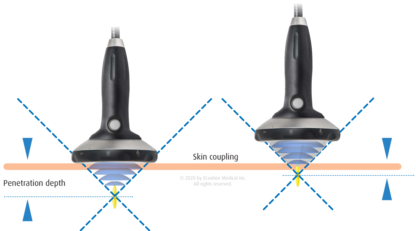
Figure 9 - Therapy source penetration depth with different gel pads
